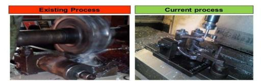
Conventional forming process replaced with VMC Milling process to achieve consistency in pad height variation
