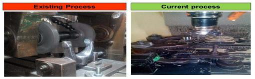
Conventional outside milling process to replaced with VMC Facing process to achieve consistency on pad thickness
